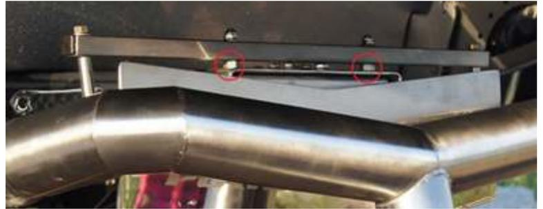
The square tube will need to be raised above the two bolts in the middle. We have supplied two nuts that are large than the bolts. These nuts are simply placed over the bolt (see red circles in drawing). You can mount the bolts facing upwards or downwards.
