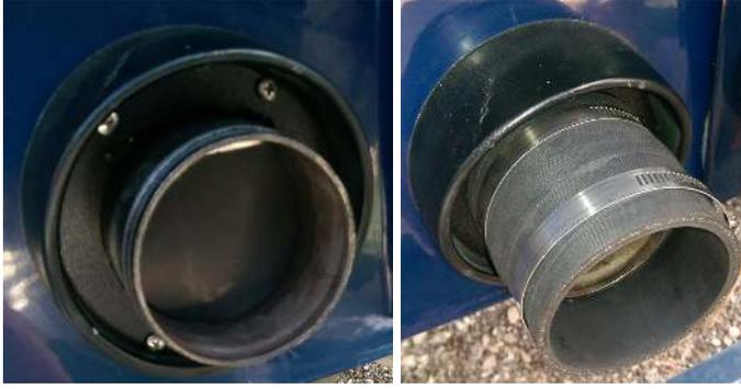
Now remove the flapper and replace with the FAE flange. Use sealant on all 4 screws and tighten. Next install the rubber hose and 2 hose clamps but leave the outer clamp loose.
