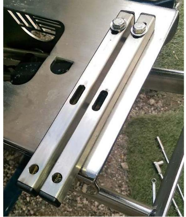
Before installing the FAE, remove the 2 port bolts only from the square tube. Once the bolts are removed, rotate the FAE into position and replace the bolts and tighten as before.
