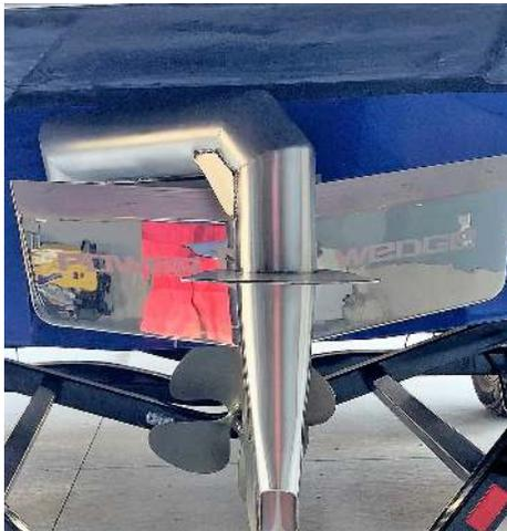
FAE bolted onto the wedge housing with the downpipe vertical and centered.
