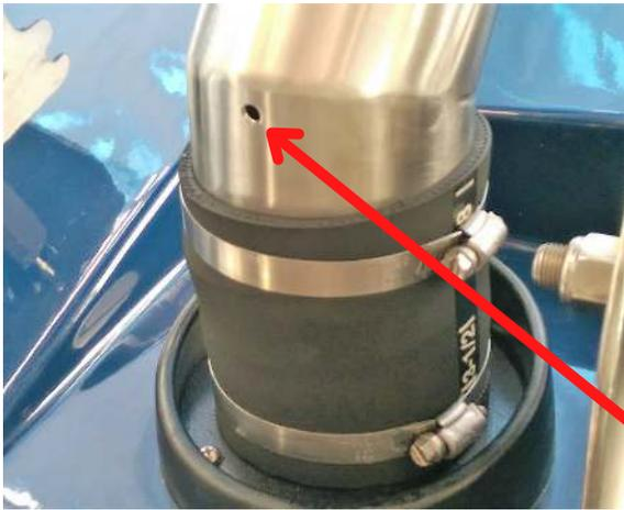
Position the hose clamps as shown in this picture with the screw heads facing down and on the inside (towards the center of the boat - they just look better there). You will need to tighten them with a 5/16" nut driver or socket; a screwdriver may not be tight enough.
