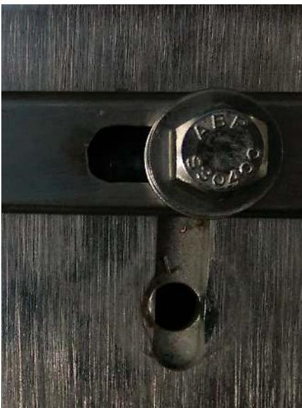
You will install the four longer bolts through the square tubes. Use the packet of anti-seize grease on the bolt threads. It is messy but will minimize the bolt from locking up.
